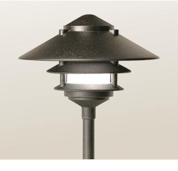
The FX Luminaire DR is one of our most popular path lights. The oversized top keeps light directed downward for controlled pathway and plant illumination without objectionable glare. The DR is constructed from die-cast aluminum alloy, and the riser is milled from solid T-6 6062 aluminum alloy for corrosion resistance and strength. The DR incorporates a halogen lamp assembly for high output and long life, reducing operating and maintenance costs.
