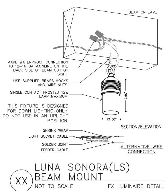
FX LUMINAIRE LUNA SONORA HANG WITH CABLE TIE. CINCH CABLE SO IT IS LOOSE TO ALLOW TREE GROWTH. REPLACE CABLE TIE EACH TIME LAMP IS REPLACED.
