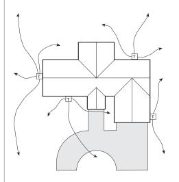
Sample diagram of home with transformer and fixture placement
