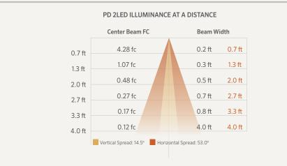
Beam angle is calculated using LM-79 method for SSL Luminaires: "Beam angle is defined as two times the vertical angle at which the intensity is 50% of the maximum."
