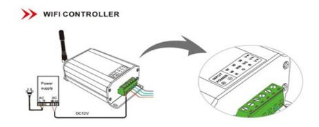
Step1: Connect Power supply (12V DC) to Input Power(DC+, DC-) of LED WIFI controller
