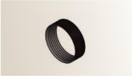
To reduce glare to a minimum specify the RecessorRing option for the MU, LO and TE. This alloy unit fits inside the fixture housing (in front of the lamp) recessing it back away from the fixture opening thereby internally cutting off glare. **RRMR16**
