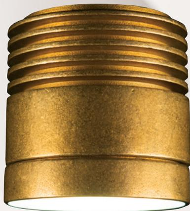
*The PS truly represents the next generation of fixed-mount LED down lights. It is meant for top-mounting, and is available with an optional copper cover. It works with 1, 3, 6 or 9LED boards and comes in all of our metal and powder coat finishes. The PS also includes a free mounting bracket that allows for tool-free servicing after initial installation.*
