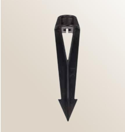
This 8" spike is the standard for all FX up lights and small path lights. Constructed from UV resistant ABS it incorporates a composite thread insert featuring a slot cut out of the threads for your wires. **SSS: 753900**
