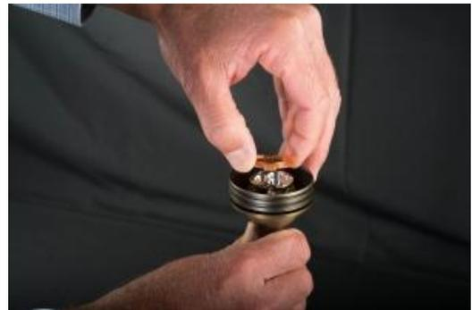
With the upper reflector now removed you can apply the same technique from the previous step to the removal of the color filter. An amber filter is shown in this demonstration.
