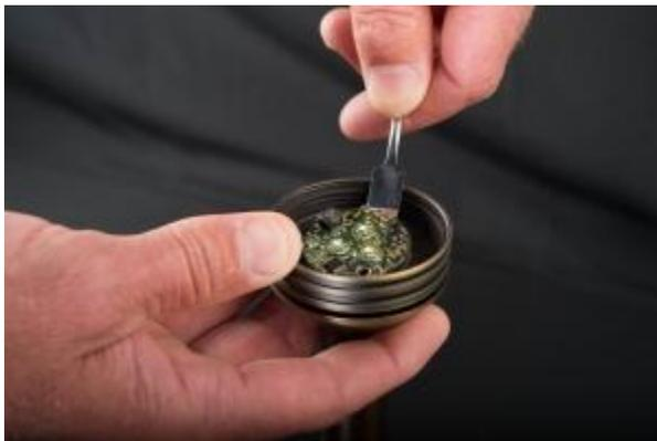
The LED board can now be removed. Using a small flat bladed screwdriver pry up gently on one side of the board taking into account the two pins on the bottom of the board. Make sure the base of the fixture where the LED was removed from is clear of debris or residual thermal pad material.
