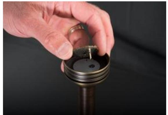
Once the LED is successfully removed this procedure can be performed backwards to install the replacement board. Replacement boards will have to be the same size LED to fit properly. All new FX LED boards come with a clear plastic coating on the back of the thermal pad, this must be removed prior to installation.
