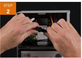
Twist the two sides of the fuse holder in opposite directions to open.
