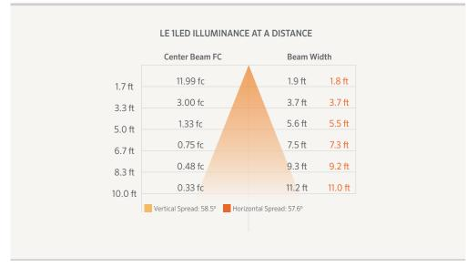
Beam angle is calculated using LM-79 method for SSL Luminaires:
