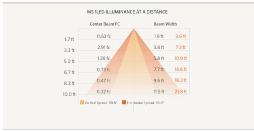
Beam angle is calculated using LM-79 method for SSL Luminaires:
