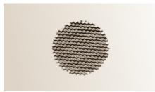
The alloy honeycomb Hex Baffle fits inside the lens cap of all FX spotlight fixtures to internally cut off light spill to 45°. 250015260000 (MR16) 250015250000 (MR11)
