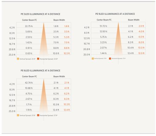
Beam angle is calculated using LM-79 method for SSL Luminaires:
