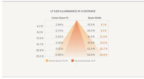
Beam angle is calculated using LM-79 method for SSL Luminaires:
