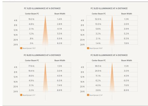
Beam angle is calculated using LM-79 method for SSL Luminaires:
