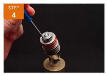
Remove the two screws holding the reflector to the fixture.
