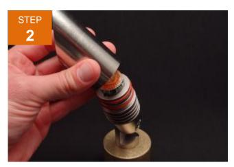
Remove the top shroud from the fixture.
