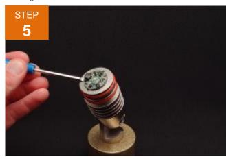
The LED board can now be removed. Using a small soft edged pry device gently pry up on one side of the board. Make sure the base of the fixture where the LED was removed from is clear of debris or residual thermal pad material.
