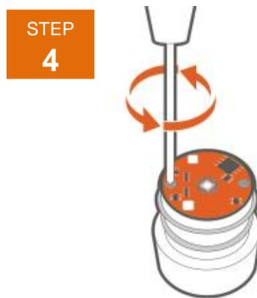
Remove the two screws holding the LED board to the lens assembly.
