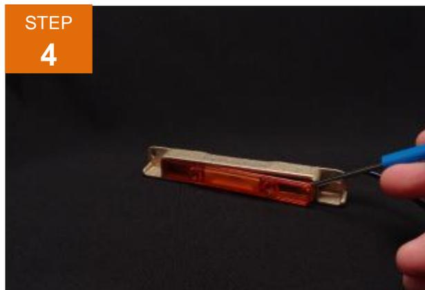
Gently pry the lens away from the housing, being careful not to damage the O-ring behind the lens.
