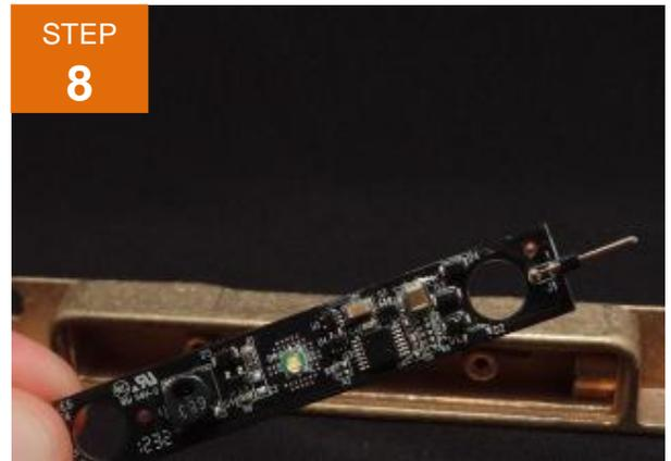
Once the LED is successfully removed this procedure can be performed backwards to install the replacement board. Replacement boards will have to be the same size LED to fit properly. All new FX LED boards come with a clear plastic coating on the back of the thermal pad; this must be removed prior to installation.
