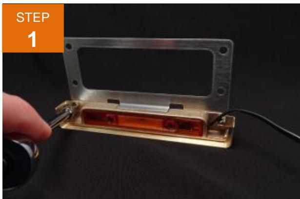
It's always a good idea to change LED boards and lamps with power to the fixture turned off completely. The LF LED fixture has two acorn nuts attaching the brass housing to mounting plate. Remove the two acorn nuts using a 5/16" socket.
