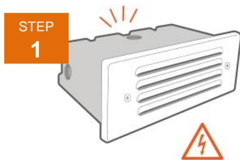
Turn off power to the fixture completely before changing the LED board in any fixture.
