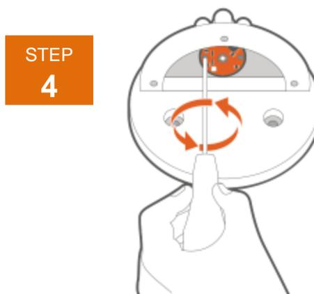
Remove the two screws holding LED board in place.
