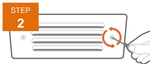
Remove the cover of the wall light with a 3/32 hex key
