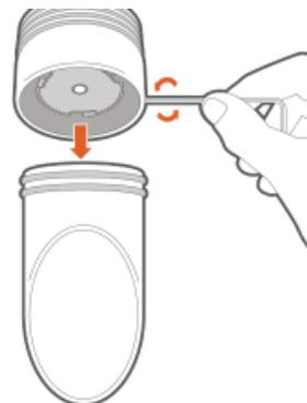
Remove the lens and shroud by loosening the set screw using a hex key 5/64 and pulling off the shroud.
