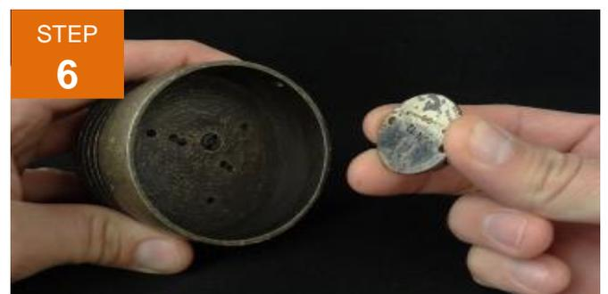
Remove the clear plastic backing from the new LED board. Insert the two metal pins into the small socket holes and gently press the board flush with the fixture base. Realign the reflector correctly over the LED diodes and refasten the small Philips screws. Replace the filters. Ensure the lens assembly is concentrically aligned over the fixture. Align the allen screw (3/32) at the top of the fixture over main housing. Firmly tighten the screw to ensure the LED board is completely sealed.
