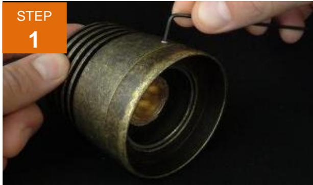
Turn off power to the transformer completely prior to disassembling the fixture. To remove the cap and lens, carefully loosen the Allen screw (3/32) on the fixture.
