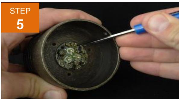
Remove the LED board using a small flat head screwdriver, gradually prying a section of the board and repeating this process around the perimeter of the board. Clear all debris or residual thermal pad material from the fixture base.
