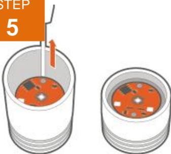
The LED board can now be removed. Using a small soft edged pry device gently pry up on one side of the board. Make sure the base of the fixture where the LED was removed is clear of debris or residual thermal pad material.
