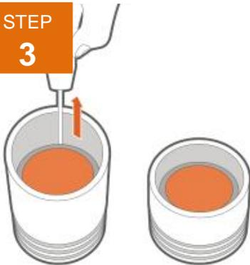
Remove any filters from the fixture by gently using a soft edged device to remove the filters and expose the LED boards.
