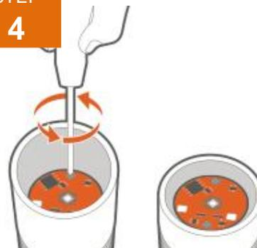
Remove the screws holding the LED board in place.
