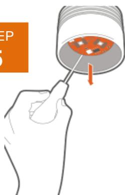
The LED board can now be removed. Using a small soft edged pry device gently pry up on one side of the board. Make sure the base of the reflector where the LED was removed is clear of debris or residual thermal pad material.
