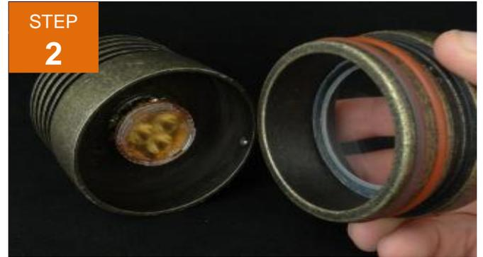
Remove the cap and lens by pulling downward to access the LED board and filters. There are O-rings on the lens cap, it may be tight to pull out.
