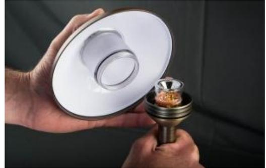
After carefully removing the top assembly you should now be able to see the reflector and filter that sit on top of the LED board
