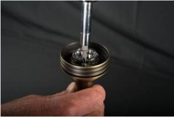
Depending on the size of the LED board, you will have two to three Phillips head screws that need to be removed to access the LED board below the reflector. Carefully remove these screws by turning each counter clockwise.
