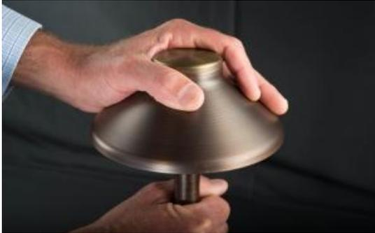
It's always a good idea to change LED boards and lamps with power to the fixture turned off completely. On FX LED fixtures the top assembly screws off counter-clockwise. Be sure to grab the riser while doing this, insuring the mounting spike doesn't move during the procedure
