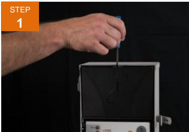
Use a flat bladed screw driver to remove cover.
