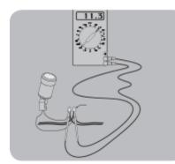
Checking voltage at fixtures
