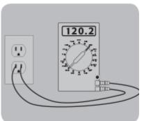
Checking voltage at plug
