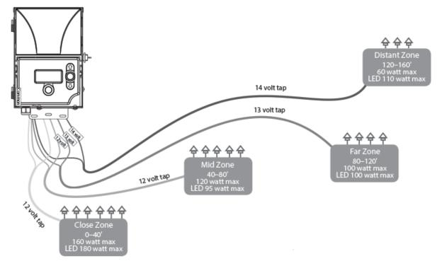
Wattages shown are per 12 gauge cable. Install additional cable runs as needed to complete project. To increase wattage maximum, run 8 gauge or double 12 gauge to the first fixture in the zone. Use a digital voltmeter to fine tune circuits.
