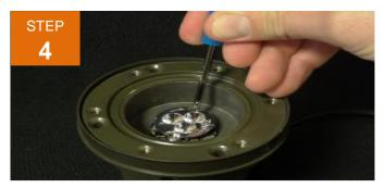
Depending on the size of the LED board, two or three Phillips head screws are required to be removed to access the LED board. Carefully remove these screws by turning each counter clockwise.
