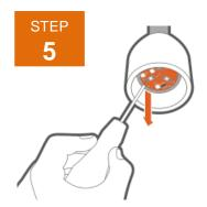
The LED board can now be removed. Using a small soft edged pry device gently pry up on one side of the board. Make sure the base where the LED was removed is clear of debris or residual thermal pad material.
