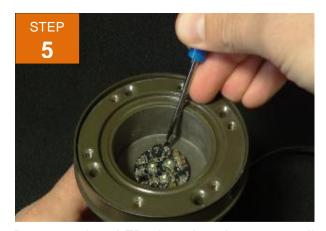
Remove the LED board using a small flat head screwdriver, gradually prying a section of the board and repeating this process around the perimeter of the board. Clear all debris or residual thermal pad material from the fixture base.
