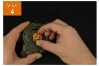
To remove the KG lens cover assembly, remove the six screws in front of fixture by turning The filter can be removed easily by turning counter clockwise.
