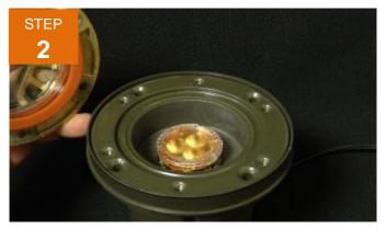
Remove the faceplate and lens assembly by lifting upward
