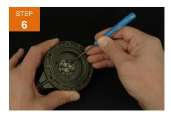
The LED board can now be removed. Using a small flat bladed screwdriver to pry outward gently on one side of the board taking into account the two pins on the bottom. Make sure the base of the fixture where the LED was removed from is clear of debris or residual thermal pad material.
