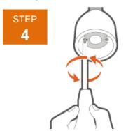
Remove the two screws holding the reflector and the LED board to the fixture using a small Phillips screwdriver.
