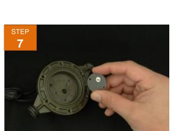
Once the LED is successfully removed this procedure can be performed backwards to install the replacement board. Replacement boards will have to be the same size LED to fit properly. All new FX LED boards come with a clear plastic coating on the back of the thermal pad, this must be removed prior to install. Replace the board being very careful the pins are lined up appropriately.
