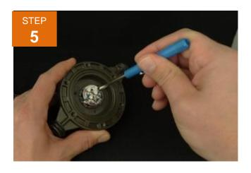
Depending on the size of the LED board, you will have two to three Phillips head screws that need to be removed to access the LED board below the reflector. Carefully remove these screws by turning each counter clockwise.
