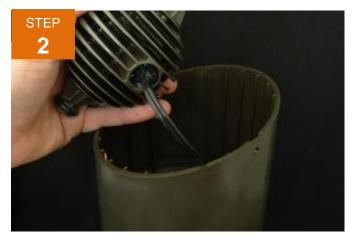
Its always a good idea to change the LED boards with power to the transformer turned off completely. To remove the KG faceplate assembly, remove the two screws on each side of fixture by turning counterclockwise using a phillips screwdriver.
