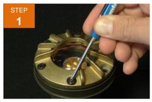
Turn off power to the transformer completely prior to disassembling the fixture. To remove the FC brass faceplate assembly, remove the six screws along the side of fixture by turning the screws counterclockwise using a Philips screwdriver.
