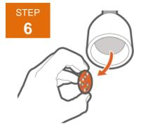
Once the LED is successfully removed this procedure can be performed backwards to install the replacement board. Replacement boards will have to be the same size LED to fit properly. All new FX LED boards come with a clear plastic coating on the back of the thermal pad; this must be removed prior to installation.
