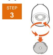
Remove the filter from the fixture by twisting it counter-clockwise and lifting it off
