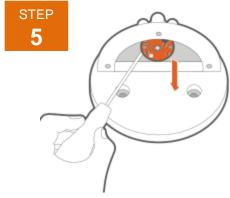
The LED board can now be removed. Using a small soft edged pry device gently pry up on one side of the board. Make sure the base of the reflector where the LED was removed is clear of debris or residual thermal pad material.
