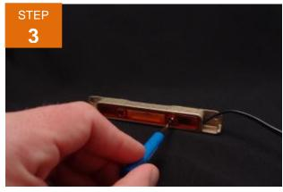
Remove the two Phillips screws from lens.
