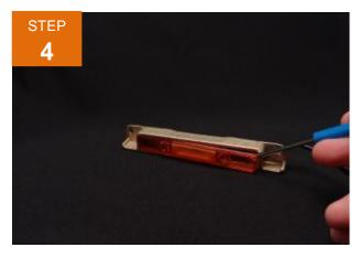
Gently pry the lens away from the housing, being careful not to damage the O-ring behind the lens.
