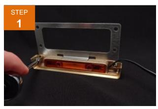
It's always a good idea to change LED boards and lamps with power to the fixture turned off completely. The LF LED fixture has two acorn nuts attaching the brass housing to mounting plate. Remove the two acorn nuts using a 5/16" socket.
