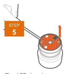
The LED board can now be removed. Using a small soft edged pry device gently pry up on one side of the board. Make sure the base where the LED was removed is clear of debris or residual thermal pad
