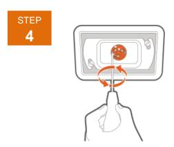
Remove the two screws holding the LED board to the fixture.
