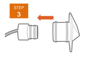
Remove the lens assembly by pulling from the faceplate.
