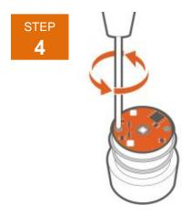
Remove the two screws holding the LED board to the lens assembly.
