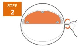
Remove the faceplate by loosening the set screws on each side of the faceplate using
