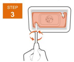
Remove any filters from the reflector by loosening the screws holding the reflector and filter in place and remove the filter.
