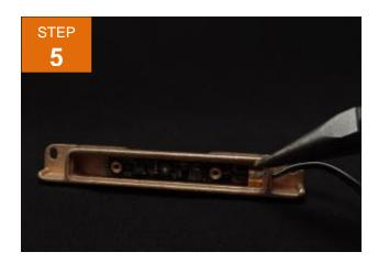
Remove the socket clip holding the socket in the housing with needle nose pliers.
