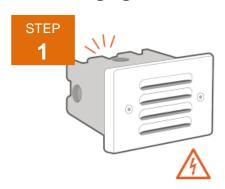
Turn off power to the fixture completely before changing the LED board in any fixture.
