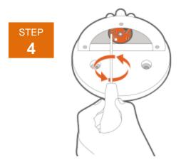
Remove the two screws holding LED board in place.
