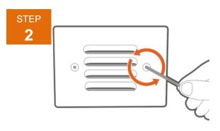
Remove the cover of the wall light with a 3/32
