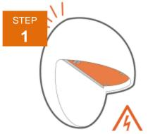
Turn off power to the fixture completely before changing the LED board in any fixture.
