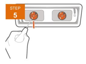
The LED board can now be removed. Using a small soft edged pry device gently pry up on one side of the board. Make sure the base of the reflector where the LED was removed is clear of debris or residual thermal pad material.
