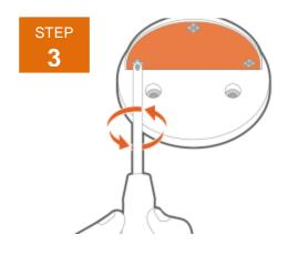
Remove the filter and the gasket by removing the 3 screws.
