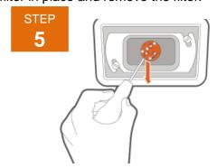
The LED board can now be removed. Using a small soft edged pry device gently pry up on one side of the board. Make sure the base of the reflector where the LED was removed is clear of debris or residual thermal pad material.
