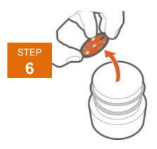
Once the LED is successfully removed this procedure can be performed backwards to install the replacement board. Replacement boards will have to be the same size LED to fit properly. All new FX LED boards come with a clear plastic coating on the back of the thermal
