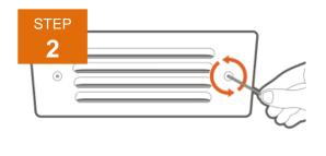
Remove the cover of the wall light with a 3/32 hex key
