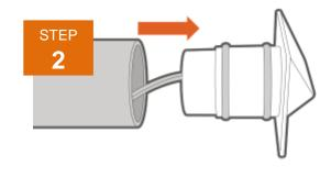
Remove the faceplate assembly by pulling it out of the sleeve.
