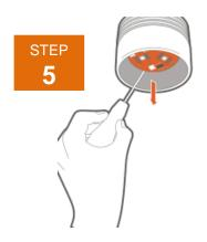
The LED board can now be removed. Using a small soft edged pry device gently pry up on one side of the board. Make sure the base of the reflector where the LED was removed is clear of debris or residual thermal pad material.
