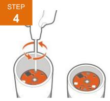
Remove the screws holding the LED board in place.
