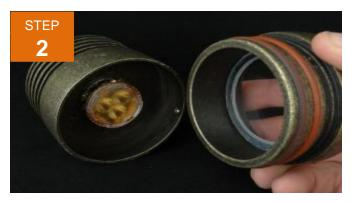
Remove the cap and lens by pulling downward to access the LED board and filters. There are Orings on the lens cap, it may be tight to pull out.
