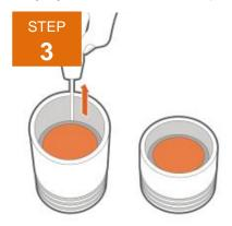
Remove any filters from the fixture by gently using a soft edged device to remove the filters and expose the LED boards.
