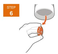
Once the LED is successfully removed this procedure can be performed backwards to install the replacement board. Replacement boards will have to be the same size LED to fit properly. All new FX LED boards come with a clear plastic coating on the back of the thermal pad; this must be removed prior to installation.
