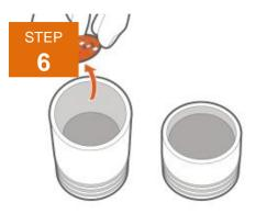
Once the LED is successfully removed this procedure can be performed backwards to install the replacement board. Replacement boards will have to be the same size LED to fit properly. All new FX LED boards come with a clear plastic coating on the back of the thermal pad; this must be removed prior to installation.
