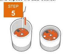
The LED board can now be removed. Using a small soft edged pry device gently pry up on one side of the board. Make sure the base of the fixture where the LED was removed is clear of debris or residual thermal pad material.
