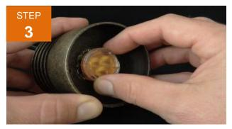
Turn the filters counter clockwise and pull up to remove
