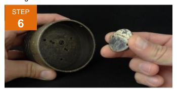
Remove the clear plastic backing from the new LED board. Insert the two metal pins into the small socket holes and gently press the board flush with the fixture base. Realign the reflector correctly over the LED diodes and refasten the small Philips screws. Replace the filters. Ensure the lens assembly is concentrically aligned over the fixture. Align the allen screw (3/32) at the top of the fixture over main housing. Firmly tighten the screw to ensure the LED board is completely sealed.
