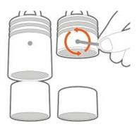
Loosen the set screw holding the reflector or shroud on the light using a 5/64 hex key and remove it.
