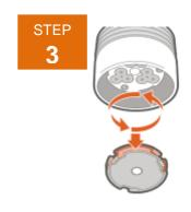
Remove any filters from the reflector by turning the filters counter-clockwise and lifting them off of the reflector.
