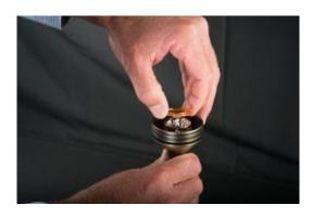
With the upper reflector now removed you can apply the same technique from the previous step to the removal of the color filter. An amber filter is shown in this demonstration.
