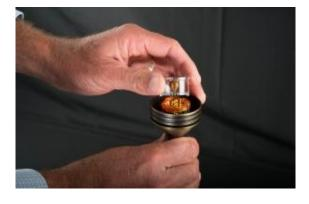
The upper reflector unlocks with a very small counter clockwise rotation.
