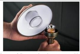
After carefully removing the top assembly you should now be able to see the reflector and filter that sit on top of the LED board
