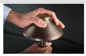
It's always a good idea to change LED boards and lamps with power to the fixture turned off completely. On FX LED fixtures the top assembly screws off counter-clockwise. Be sure to grab the riser while doing this, insuring the mounting spike doesn't move during the procedure
