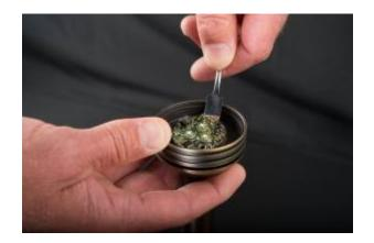
The LED board can now be removed. Using a small flat bladed screwdriver pry up gently on one side of the board taking into account the two pins on the bottom of the board. Make sure the base of the fixture where the LED was removed from is clear of debris or residual thermal pad material.
