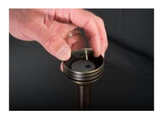
Once the LED is successfully removed this procedure can be performed backwards to install the replacement board. Replacement boards will have to be the same size LED to fit properly. All new FX LED boards come with a clear plastic coating on the back of the thermal pad, this must be removed prior to installation.
